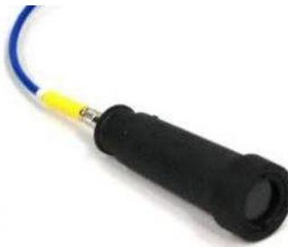
Figure 2: Fiber Optic Collimator
