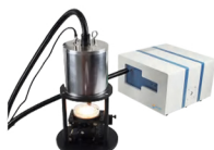
Non-Contact Diffuse Reflection Measurement of Powder Samples
