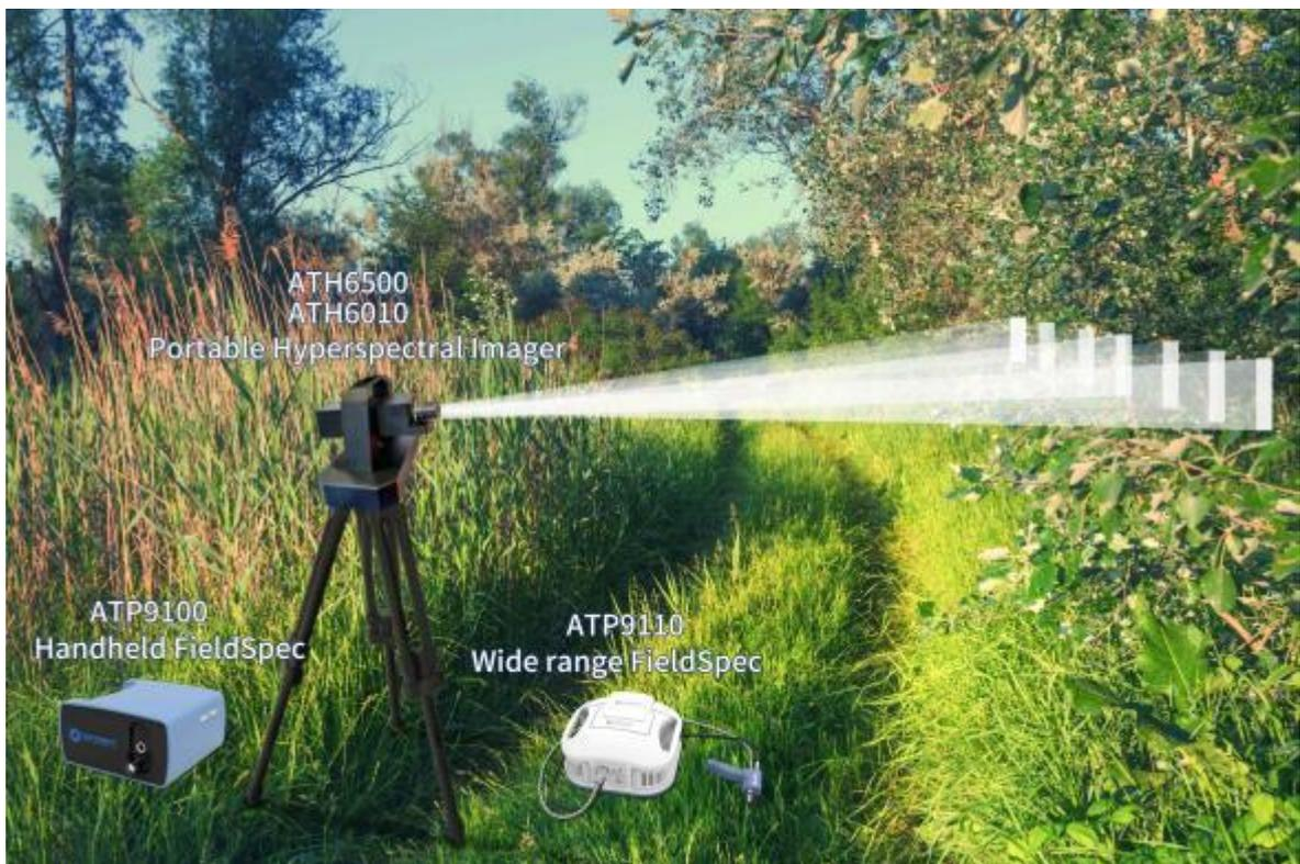
Figure 1 The cooperative use of FieldSpec spectroradiometers and hyperspectral imager.
