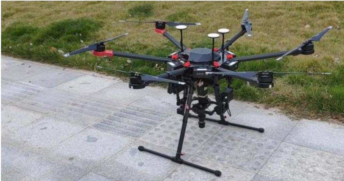
Figure 16 Drone-borne hyperspectral imaging camera
