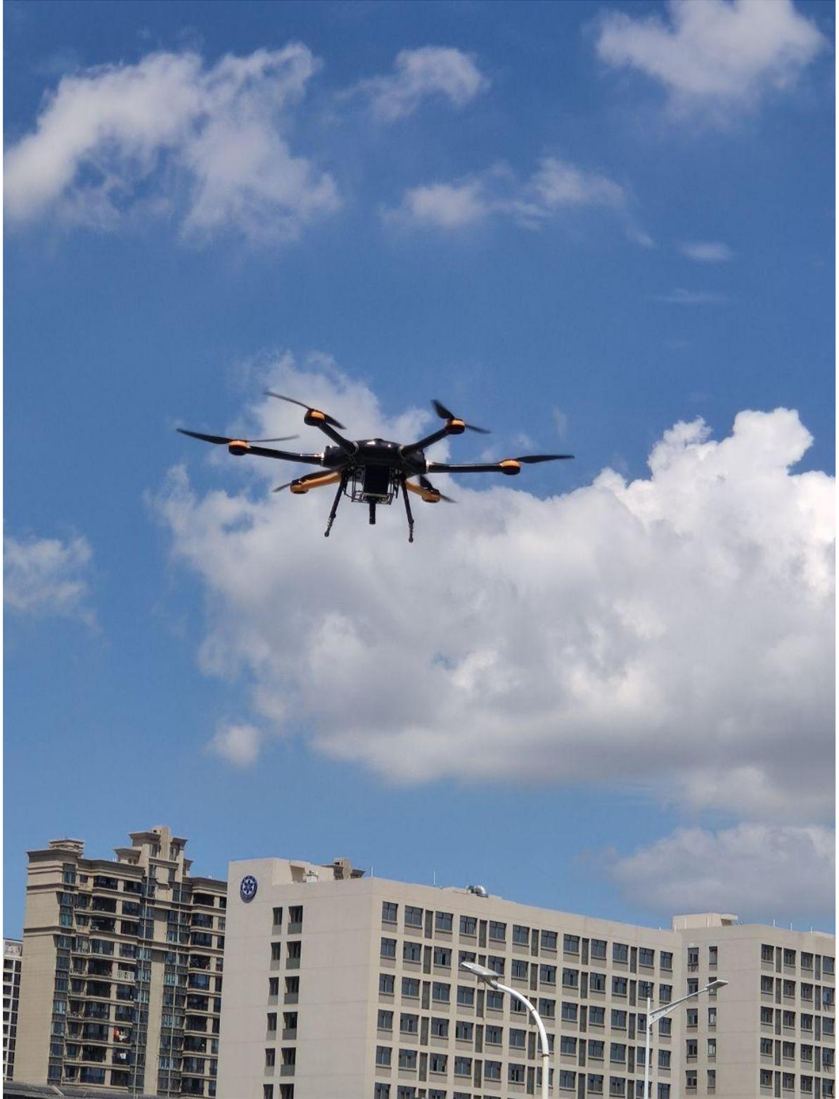
Fig 8 ATH9010 series UAV-borne hyperspectral imager
