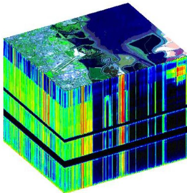
Fig 5 Data cube captured by hyperspectral imager
