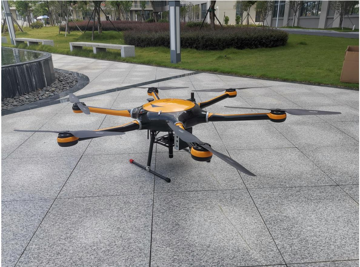
Fig 7 ATH9010 series UAV-borne hyperspectral imager
