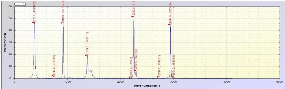
Figure 1 Raman spectrum curve test results; sample: acetonitrile, laser power: 130mW, measurement integration time: 4000ms.
