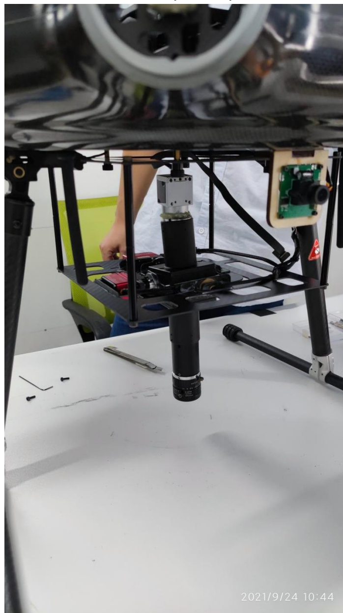
ATH1010 hyperspectral imager mounted on the drone
