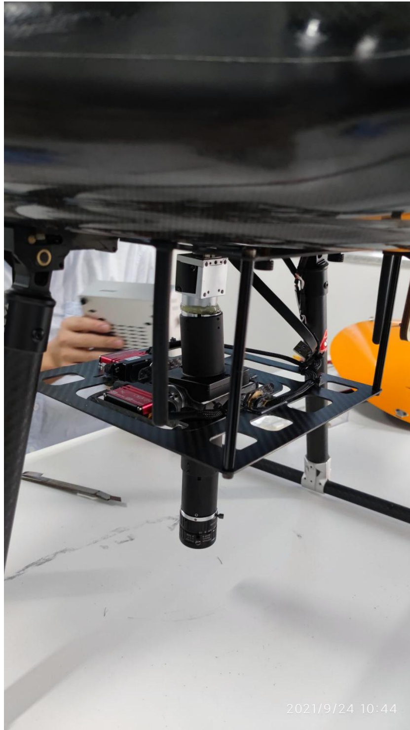
ATH1010 hyperspectral imager mounted on the drone
