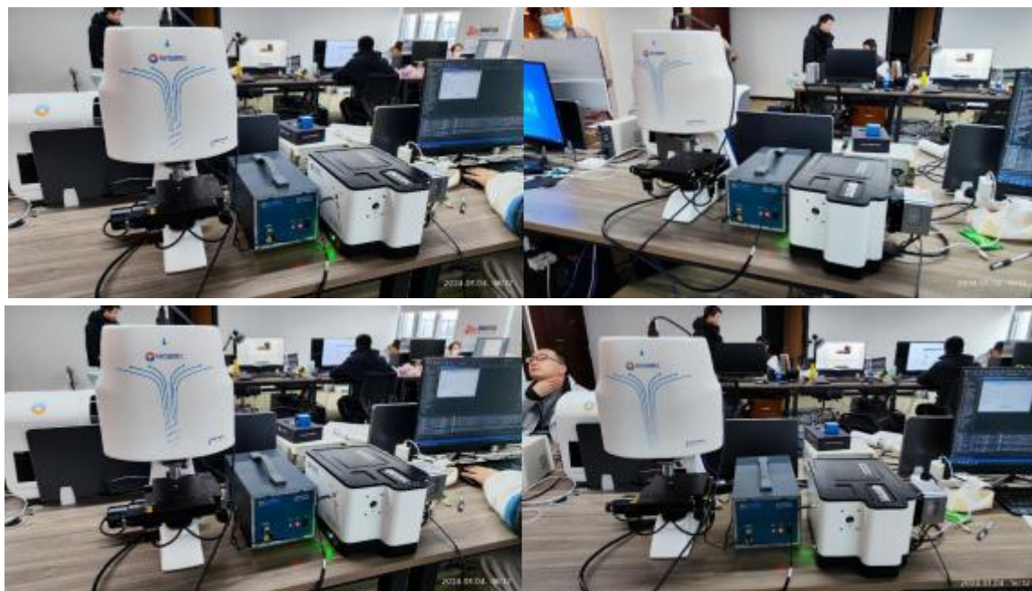
Figure 6 ATR8300Pro-FL510 high-resolution Raman microscope (focal length 510mm).
