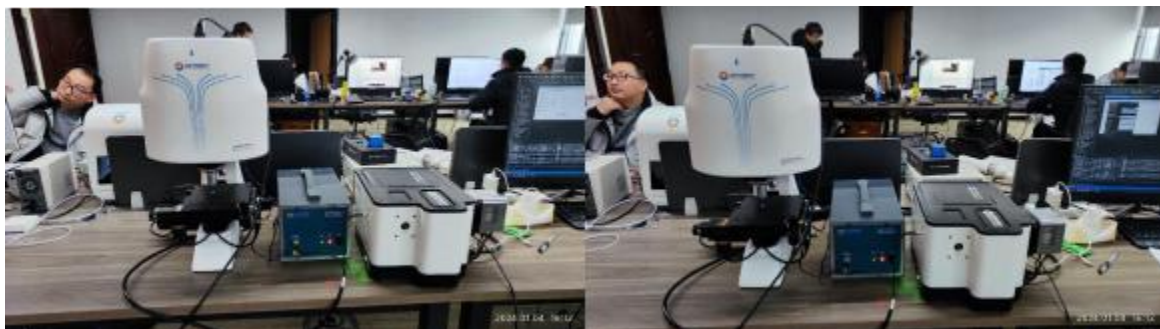
Figure 7 ATR8300Pro-FL210 high-resolution Raman microscope (focal length 210mm).
