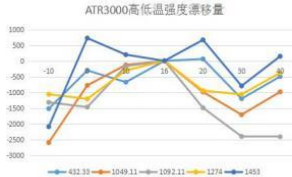
Figure 5 Intensity variation - 10 °C to 40 °C of ATR3000SJ portable Raman spectrometers, sample is alcohol.
